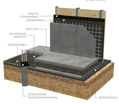
The membranes are composed of a select blend of highperformance SBS modified bitumen, an ultra-high-strength reinforcement and specially designed top surface.
