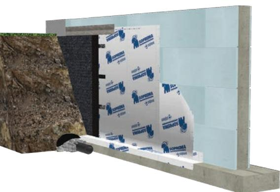
COLPHENE ICF is a high quality self-adhesive membrane composed of SBS modified bitumen and a tri-laminate woven polyethylene facer. The membrane provides damproofing and waterproofing on ICF formwork systems.
