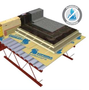
SOPRATACK is an odour-free, two-component polyurethane adhesive with very low VOC content. It is used to adhere SBS polymer modified bitumen membranes on low-slope surfaces.
