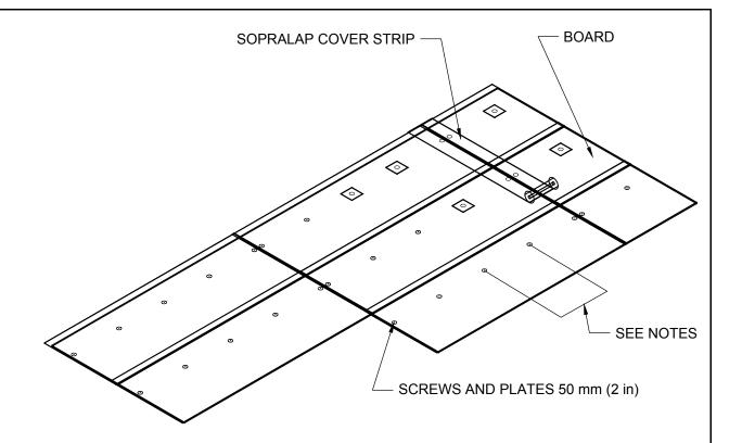
NOTE 1: SCREWS ANS PLATES ARE INSTALLED THE FIELD OF THE BOARD AND COVERED WITH A SOPRALAP COVER STRIP.
