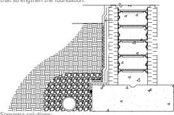
Soprema products that can be used for this type of foundation: Colphene ICF, Sopradrain 10-G, 15-G or 18-G and Sopradrain HF.
