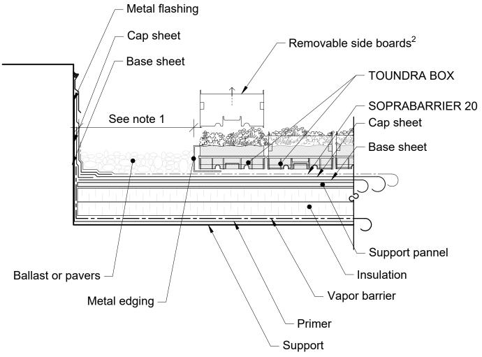
Note 1: Provide vegetation-free zone at the base of upstands, around drains and roof projections as per applicable standards. Note 2 : The side boards must be removed once the TOUNDRA BOX are installed
