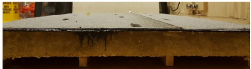
Mineral Wool Roof Specimen after Heating
