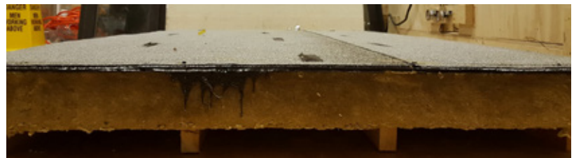
Mineral Wool Roof Specimen after Heating
