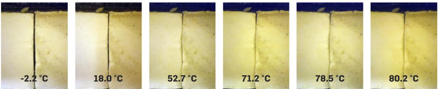
Photographs of the gap between insulation boards during exposure to uniform heating and cooling of the roof specimens.
