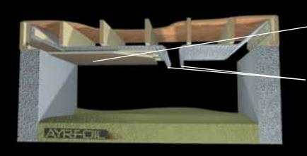
R-21 1" RIGID INSULATION AND AYR-FOIL™ A2A R-12.5 AYR-FOIL™ A2A ADDS R-4.5 TO THE R-VALUES OF WALLS
