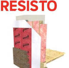
Self-adhesive vapor permeable air barrier membrane which stands out for its unmatched adhesion. It is used as an intramural membrane and as a transition membrane.
