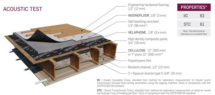
\*IIC and STC results are presented for information purpose only. Equivalent performance cannot be guaranteed by Soprema. (1): According to us, the use of 32 mm (1 ¼ in) of self-levelling concrete or use of any type of concrete will not have a significative influence on the acoustical results. (2): According to us, the use of web open ioists will not have a significative influence on the acoustical results.
