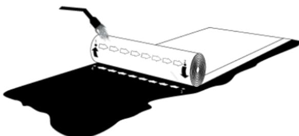
Never direct the flame between the roll and the substrate. This could trap air under the membrane and cause blisters or ridges.
