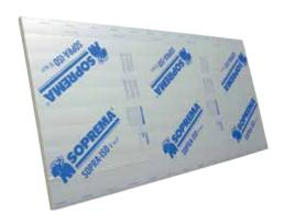
SOPRA-ISO V ALU is a closed-cell polyisocyanurate foam insulation board laminated with a radiant barrier quality reflective foil facer on the back side and a non-reflective aluminum facer on the top surface.
