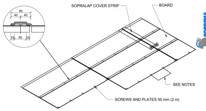
NOTE 1: SCREWS AND PLATES ARE INSTALLED WITHIN AND IN THE CENTRE OF THE LAP ONLY.
