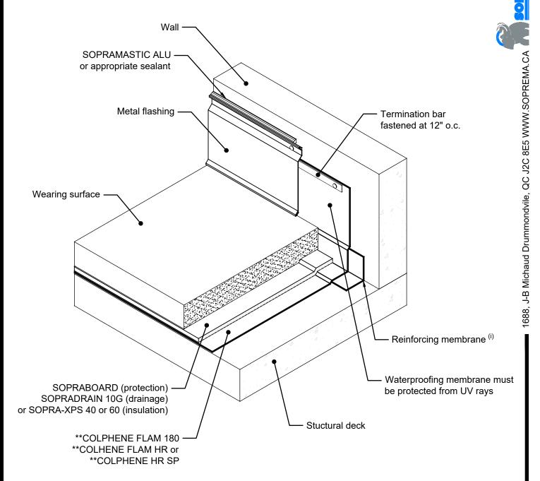
Note: Termination membranes needs to exceed minimum 4" over top wearing surface (i): Use the waterproofing membrane installed on the system as reinforcing membrane.
