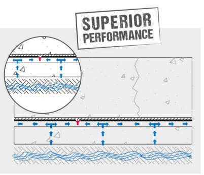
OTHER OFFERINGS ON THE MARKET: Concept of a Conventional Waterproofing System (When **not bonded** to the structural concrete slab)
