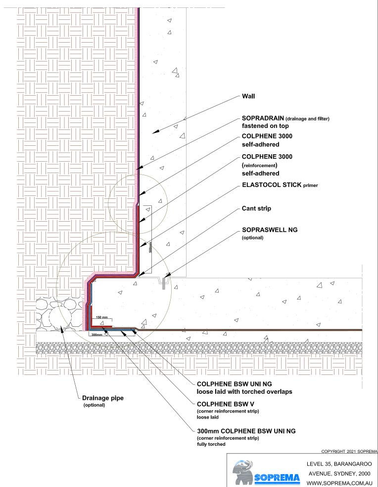
Without chamfer on all angles, a corner reinforcement must be previously applied
