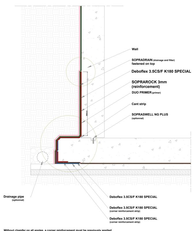
Without chamfer on all angles, a corner reinforcement must be previously applied
