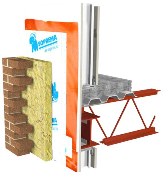
SOPRASEAL STICK 1100 T is a self-adhesive air/vapour barrier membrane for walls composed of SBS modified bitumen and a tri-laminate woven polyethylene facer. It is also used as masonry and through-wall flashing membrane as well as waterproofing membrane at openings and transitions.
