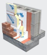
Masonry cladding can be used with SOPRA-ISO V boards. The insulation board is mechanically attached or installed with adhesive and supported by brick ties.
