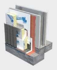
Metal cladding can be installed with SOPRA-ISO V boards using Z bars or anchoring systems with thermal breakage.
