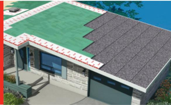
Self-adhesive base sheet membrane used in the sealing of single-ply or two-ply roofing systems.
