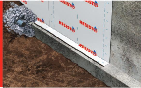
Self-adhesive waterproofing membrane composed of SBS modified bitumen and a tri-laminated woven polyethylene facer used on foundation walls.
