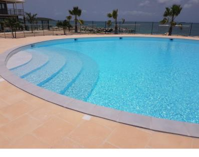
**FLAGPOOL®** is a PVC synthetic membrane reinforced with a polyester mesh, made by spreading. It is used for the internal lining of swimming pools.
