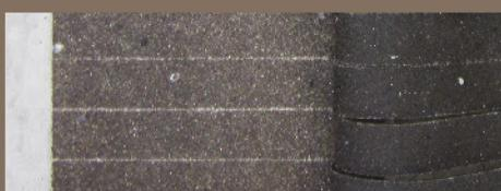
The top face of the membrane is made of SBS-modified bitumen and covered with sand. The specially formulated surface softens slightly as the concrete begins to cure, releasing heat. This contributes to the adhesion of the membrane to the concrete, and prevents the ingress or migration of water around the structure.
