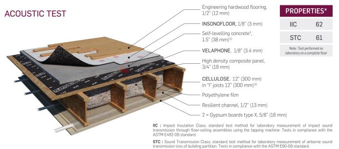
\*IIC and STC results are presented for information purpose only. Equivalent performance cannot be guaranteed by Soprema. (1): According to us, the use of 32 mm (1 ¼ in) of self-levelling concrete or use of any type of concrete will not have a significative influence on the acoustical results.
