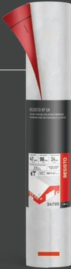
RESISTO VP SA is a self-adhesive vapor-permeable air-barrier membrane with a trilaminated polypropylene complex on its surface. Used in walls, its superior breaking and tear strength, combined with a self-adhesive underface, protected by a silicone release film, make it very easy to install. It can be used on most building surfaces such as masonry, concrete, wood, and gypsum.
