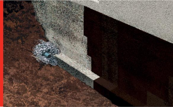
A coating composed of bitumen and fast evaporating solvent. It is used for damproofing of foundation walls, footings, retaining walls, wing walls, abutments and culverts.
