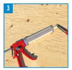
Unscrew the nozzle, cut the external applicator from the cartridge, and screw the nozzle onto it or pierce the seal if necessary. Cut the nozzle to the desired opening. It is recommended to reuse the same nozzle when changing cartridges to ensure that you have the same sealant bead thickness throughout the application.
