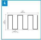
Apply the foam in 2 to 3 cm (3/4 to 1 1/8 in) wide strips, 3 cm (1 1/8 in) from the edges of the insulation board and forming a continuous "S" every  $45 \, \text{cm}$  (16 in).
