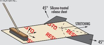
5. Continue to remove the protective film while applying pressure with the broom on the bonded portion.
