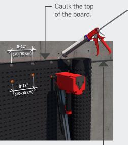
Apply a bead of caulk between the – smooth strip of the drainage board and the wall.
