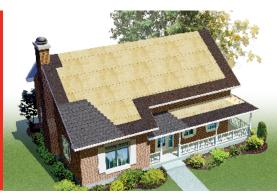
Roof underlay adhesive membrane consisting of a reinforced glass mat and sand covered surface which is slip resistant.
