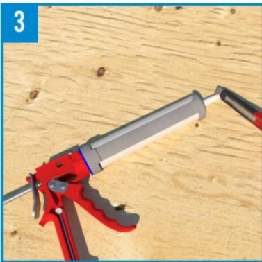
Unscrew the nozzle, cut the external applicator from the cartridge, and screw the nozzle onto it or pierce the seal if necessary. Cut the nozzle to the desired opening. It is recommended to reuse the same nozzle when changing cartridges to ensure that you have the same sealant bead thickness throughout the application.
