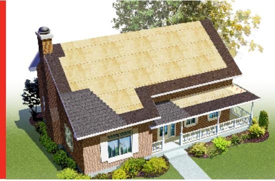
Roof underlay adhesive membrane consisting of a reinforced glass mat and sand covered surface which is slip resistant.
